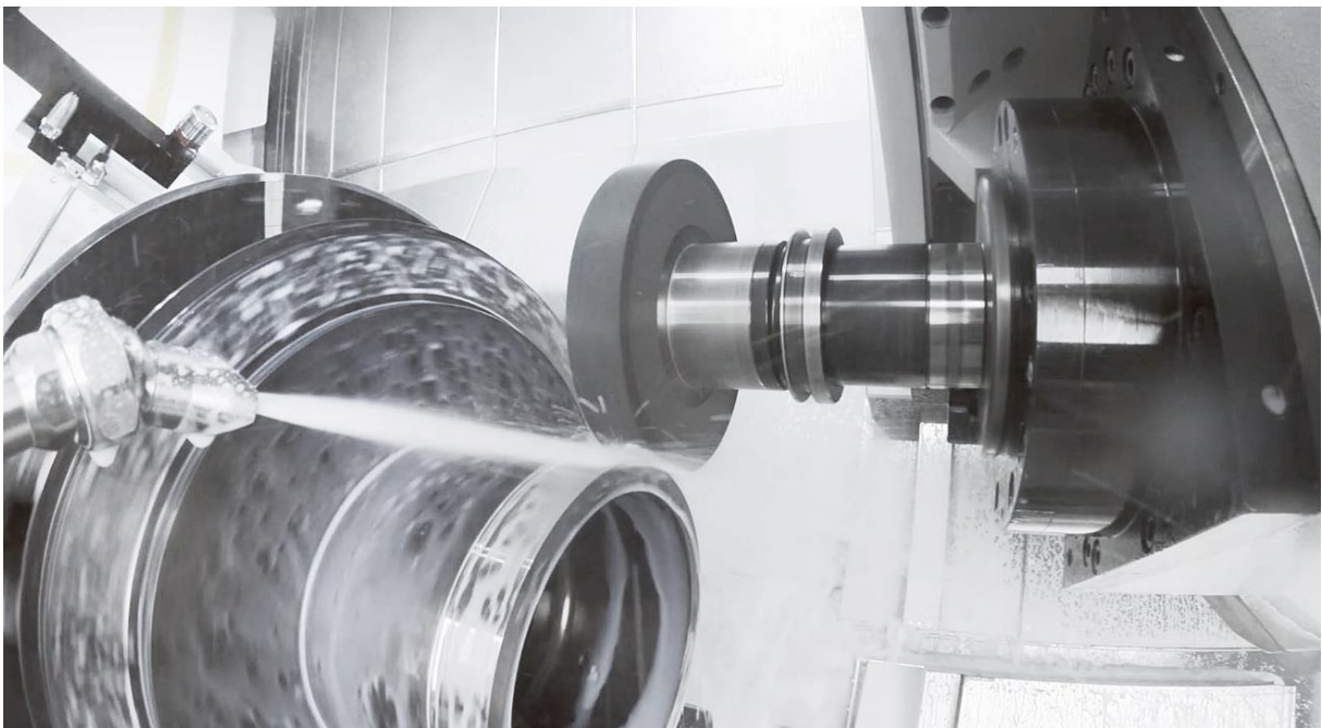
Image 5 –Process integration: Grinding including dressing unit and specific process-software
