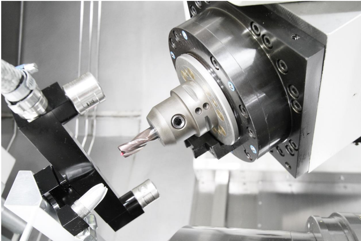
Image 3 – Integrated tool measurement with laser
