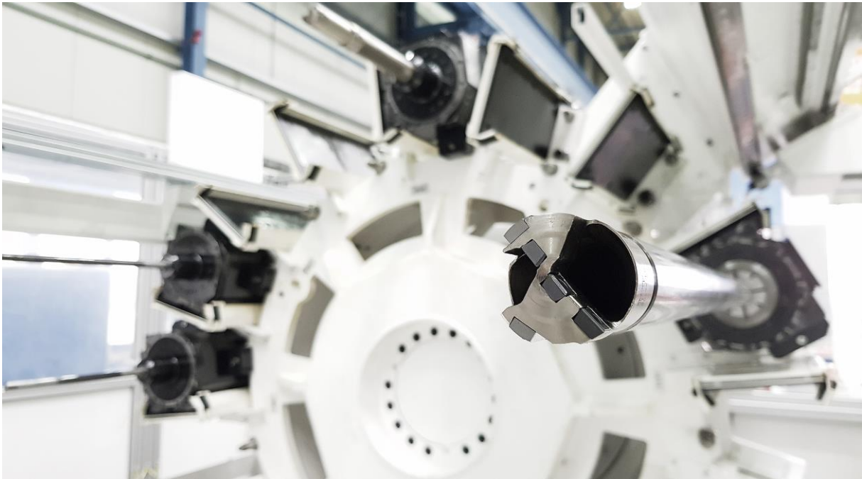
Image 4 – Additional boring bar magazine for complex internal machining
