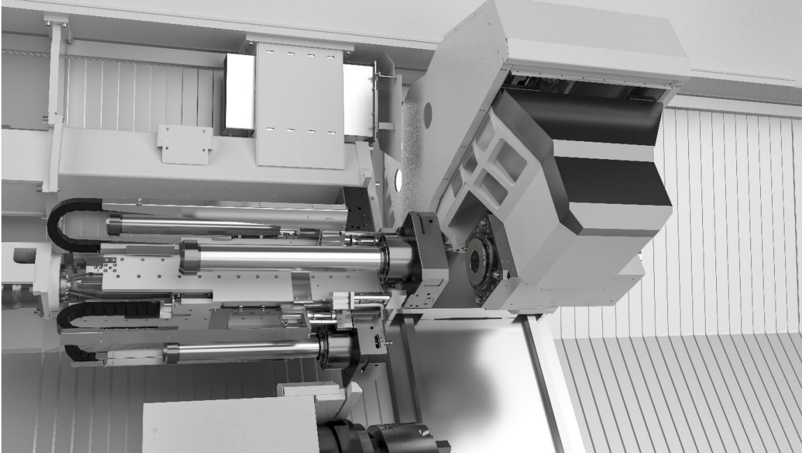
Figure 4 – Hydrodock unit with three-position pickup magazine
