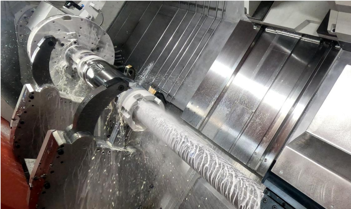
Figure 3 – Internal machining with high-pressure coolant and sensor-supported boring bars.
