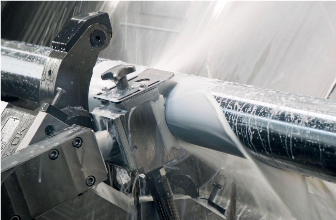
Figure 2 – TURN-MILL with hydrostatic support for excellence in shaft machining
