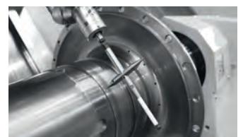
– In-Process Measuring (workpiece/tools)
