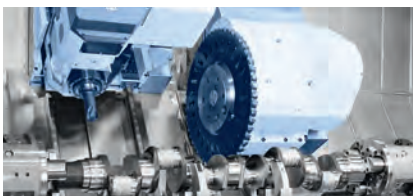
– Combination Turning-Milling-Boring Unit and External Milling Unit
