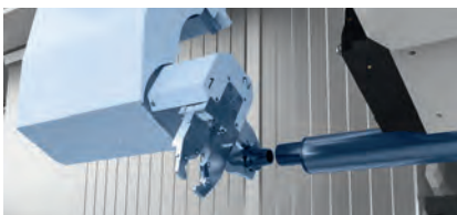
– Automatic Tool Change (ATC) for System Boring Bars
