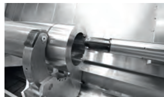
– Internal Machining with System Boring Bar or Quill
