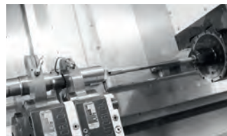
– Deep-hole Drilling | Ejector Drilling
