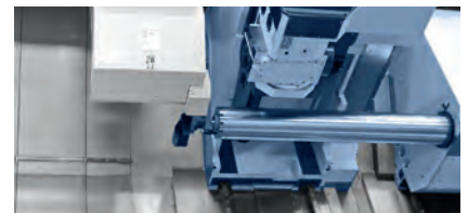
– Combination Turning-Milling-Boring Unit and Drilling Quill
