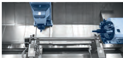
– Combination Turning-Milling-Boring Unit and Tool Carrier
